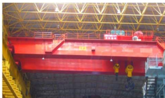
QD hook double girder gantry crane
