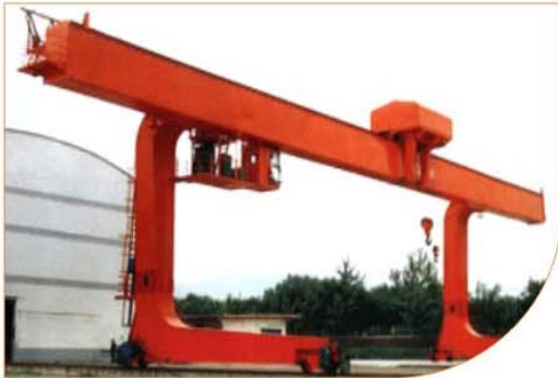
MDG hook single girder gantry crane
